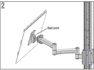
Mount VESA plate/bin rail assembly to arm by sliding the large emboss on the VESA plate over the top flange of ball joint.
