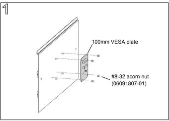
Install 100mm VESA plate (from flat screen arm) to bin rail using (4) acorn nuts provided. Tighten using a **5/16"** open end wrench.
