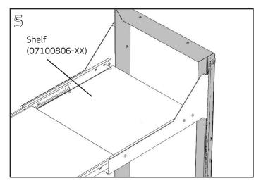
Lift rear of shelf over latch tab and align inner and outer slides. Push shelf back (toward frame) to engage slides.
