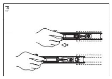
Remove outer slide from shelf. To remove slide, extend slide, pull black release tab, and pull inner and outer slides apart.
