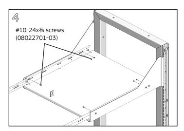
Fully extend outer shelf brackets. Align holes in slides with weldnuts on brackets. Insert #10-24x3/8 flathead screws (3 per side) using a #2 Phillips screwdriver. Completely tighten screws.
