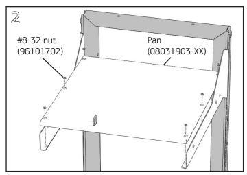
Place pan on support brackets aligning holes in pan with the threaded studs on the brackets. After pan is in place, start all (6) nuts by hand and tighten with 11/32 nut driver.
