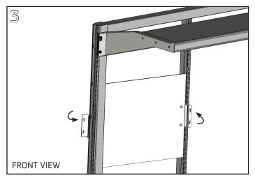
Rotate white board and insert in Riser Frame opening. Align screw heads in hanger clip with round center hole in each bracket and slide board down so top of keyslots rest on top screws. Install one #10-24x3/8" Phillips pan head screw into bottom hole on each hanger clip. Tighten all screws.
