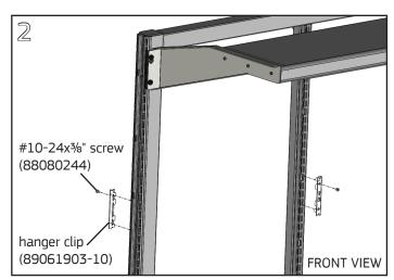
Insert a hanger clip on the back of the Riser Frame and the front of the Riser Spine at the same heights. Install one #10-24x%" Phillips pan head screw into the top threaded hole of each hanger clip using a using a #2 Phillips screwdriver, leaving leaving a 1/8" gap between head of screw and clip face.
