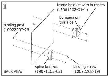
Attach brackets to holes in white board using (2) binder posts and #8-32x¾6" binder screws per bracket using a #2 Phillips screwdriver and a ¼" flat-blade screwdriver. Mount the shorter spine bracket on the Riser Spine side, and the longer frame bracket on the Riser Frame side. Note: polyurethane mounting bumpers on Riser Frame bracket should face toward the front of the white board. Left-hand Center mounting on Riser Frame is illustrated.
