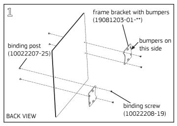
Attach brackets to holes in white board using (2) binder posts and #8-32x¾6" binder screws per bracket using a #2 Phillips screwdriver and a ¼" flat-blade screwdriver. Note: polyurethane mounting bumpers should face away from white board.
