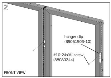
Insert a hanger clip on each side of the UltraFrame at the same heights. Install one #10-24x¾" Phillips pan head screw into the top hold of each hanger clip using a #2 Phillips screwdriver, leaving leaving a ⅓" gap between head of screw and clip face.
