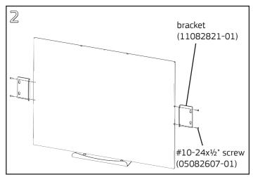
Attach brackets to side threaded inserts with (2) #10-24x½" flathead screws per bracket using a **#2 Phillips screwdriver**.
