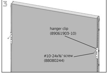
Insert a hanger clip on each side of the panel at the same heights. Install one #10-24x3% Phillips pan head screw into the top hole of each hanger clip using a #2 Phillips screwdriver, leaving a 1/8 gap between head of screw and clip face.
