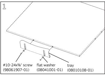
Attach tray to bottom threaded inserts with (2) flat washers and (2) #10-24x%" Phillips pan head screw using a **#2 Phillips screwdriver**. Adjust position so that the back lip of the tray touches the back of the white board.
