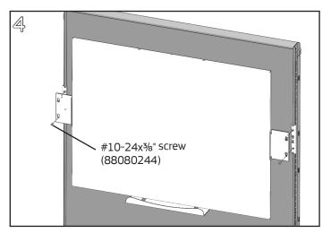
Align screw heads in hanger clips with round center hole in each bracket and slide board down so top of keyslots rest on top screws. Install one #10-24x3/8" Phillips pan head screw into bottom hole on each hanger clip. Tighten all screws.
