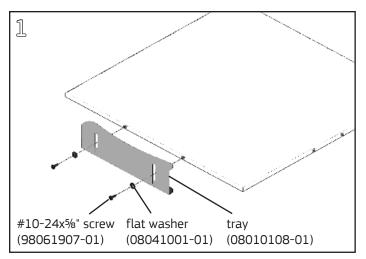
Attach tray to bottom threaded inserts with (2) flat washers and (2) #10-24x%" Phillips pan head screw using a **#2 Phillips screwdriver**. Adjust position forward or backward to desired location before fully tightening screws.
