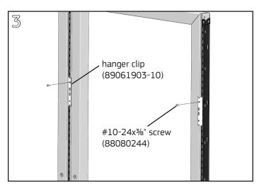
Insert a hanger clip on each side of the UltraFrame at the same heights. Install one #10-24x3/8" Phillips pan head screw into the top hole of each hanger clip using a **#2 Phillips screwdriver**, leaving a 1/8" gap between head of screw and clip face.
