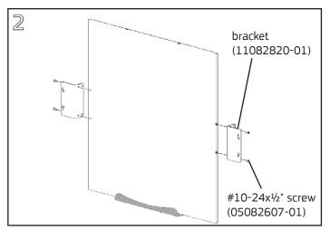
Attach brackets to side threaded inserts with (2) #10-24x½" flathead screws per bracket using a **#2 Phillips screwdriver**. White board can be mounted flush with the front of the frame or centered in the frame. Flush mounting is shown.
