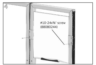
Align screw heads in hanger clip with round center hole in each bracket and slide board down so top of keyslots rest on top screws. Install one #10-24x<sup>3</sup>/<sub>8</sub>" Phillips pan head screw into bottom hole on each hanger clip. Tighten all screws.
