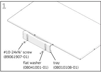
Attach tray to bottom threaded inserts with (2) flat washers and (2) #10-24x%" Phillips pan head screws using a **#2 Phillips screwdriver**. Adjust position forward or backward to desired location before fully tightening screws.
