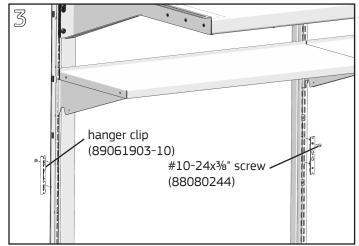
Insert a hanger clip on the back of the Riser Frame hanger frame and the front of the Riser Spine at the same heights. Install one #10-24x3/8" Phillips pan head screw into the top hole of each hanger clip using a #2 Phillips screwdriver, leaving an 1/8" gap between head of screw and clip face.
