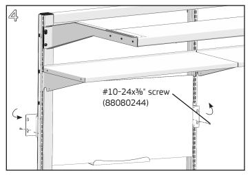
Rotate white board and insert in Riser Frame opening. Align screw heads in hanger clip with round center hole in each bracket and slide board down so top of keyslots rest on top screws. Install one #10-24x3%" Phillips pan head screw into bottom hole on each hanger clip. Tighten all screws.
