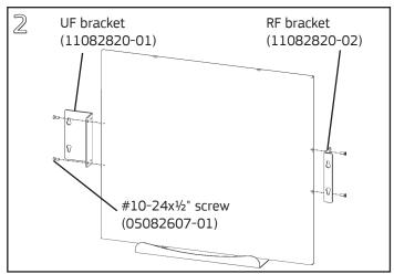
Attach brackets to side threaded inserts with (2) #10-24x½" flathead screws per bracket using a #2 Phillips screwdriver. Mount the shorter spine bracket on the Riser Spine side, and the longer frame bracket on the Riser Frame end. Left-hand Center mounting on Riser Frame is shown.
