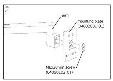
Fasten arm to mounting plate with (2) M8x20mm flathead socket drive screws using a **5mm Allen** wrench.
