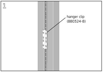
Install two hanger clips at the same height at the frame joint. Ensure clips are firmly seated in the slots.
