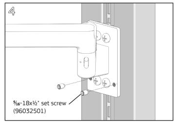
Install a \%-18x\%" set screw on each side of the mounting plate. Tighten with a **4mm Allen wrench** until the set screw tips push against the UltraFrame.
