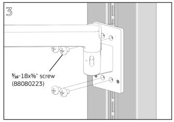
Align the four slots in the mounting plate with the threaded holes in the hanger clips. Fasten with (4) \(^{1}\)6-18x\(^{3}\)8" Phillips pan head screws using a **#4** Phillips screwdriver.
