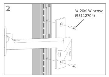
Align the countersunk holes in the mounting plate with threaded inserts in the end of the Riser Frame. Fasten with (2) ¼-20x1¼" flathead socket driver screws using a 5/32" Allen wrench.
