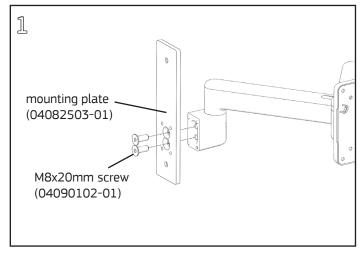
Fasten the arm to the mounting plate with (2) M8x20mm flathead socket drive screws using a **5mm Allen wrench**.
