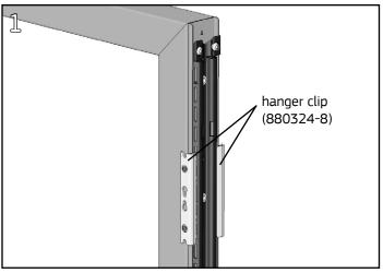
Install two hanger clips at the same height, one on the front and the other on the back of the hanger frame.
