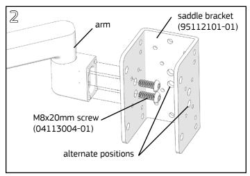
Select one of the three arm positions on the saddle bracket. Fasten arm to bracket using (2) M8x20mm socket drive screws using a **6mm Allen wrench**.
