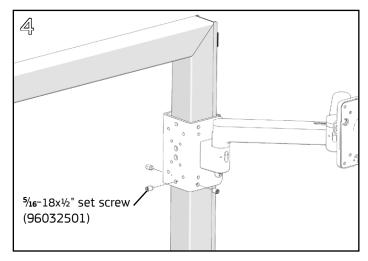
Insert (3) 16-18x½" set screws into the lower tapped holes of the saddle bracket on the front, back and inside faces. Tighten against the UltraFrame tube using a 4mm Allen wrench.
