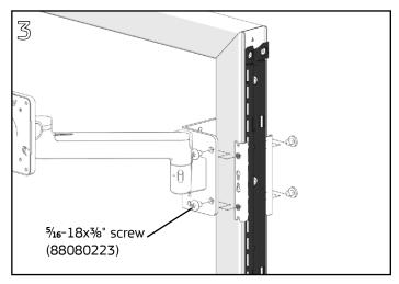
Slide the saddle bracket over the clips. Fasten saddle bracket to the weldnuts in the hanger clips with (4) \(^{1}\)6-18x\(^{3}\)8" Phillips pan head screws using a **#4 Phillips screwdriver**.
