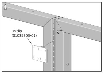
Install Uniclip into one side of the hanger frame joint at the desired height. Ensure that the clip is firmly seated in the slots.
