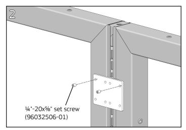
Install a ¼-20x%" set screw on both the left and right side of the clip, in either the upper or lower tapped holes. Tighten with a ¼" Allen wrench until the clip is parallel with the face of the UltraFrame. Mount components to clip as needed.
