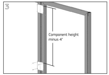
Repeat steps 1 and 2 with a second pair of Utility Mounting Brackets below the first pair. The distance from the top of the top brackets to the top of the bottom brackets needs to be 4" less than the nominal size of the component to be mounted.
