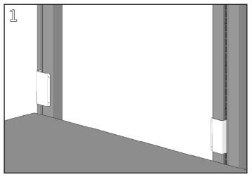
At the required mounting height, install the bracket on the left and right sides of the frame. Ensure the brackets are securely seated in the hanger frame slots
