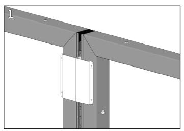
Install first bracket in the hanger frame slot at the frame joint. Install second bracket adjacent to the first at the same height. Ensure brackets are securely seated in the hanger frame slots.
