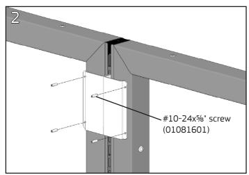
Install two #10-24x%" set screws into the tapped holes on each bracket. Tighten each set of screws with a 3/52" Allen wrench until the brackets are flush.
