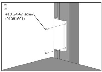
Install two #10-24x%" set screws into the tapped holes on each bracket. Tighten each set of screws with a 3/52" Allen wrench until the bracket is parallel to the front of the frame.
