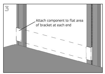
Mount component to the flat surface of each bracket using self-drilling screws with a #2 drill point (not provided). Do not screw into the flange with set screws. Screw length must not exceed 3/4".
